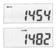
When there is no activity, and no counts are made the display automatically switches between both directions.
