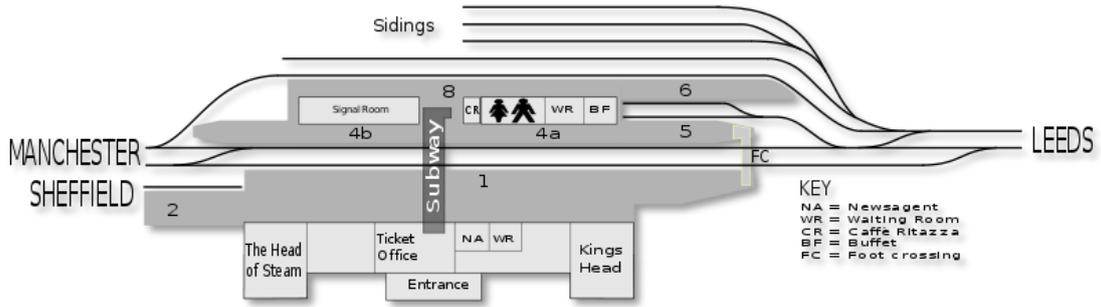
Figure 2 shows the plan of the station. The PM peak trains arriving from Leeds detrain onto Platform 1 and exit above the area marked 'Subway'. A 1.12m exit and a 1.2m wide exit are provided, which generate a queue condition for busy periods.
